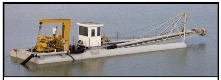
10" H-Series dredge with rotary cutter ladder.
