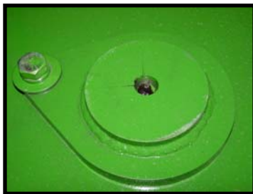
Extreme duty shaft with recessed grease zerks.
