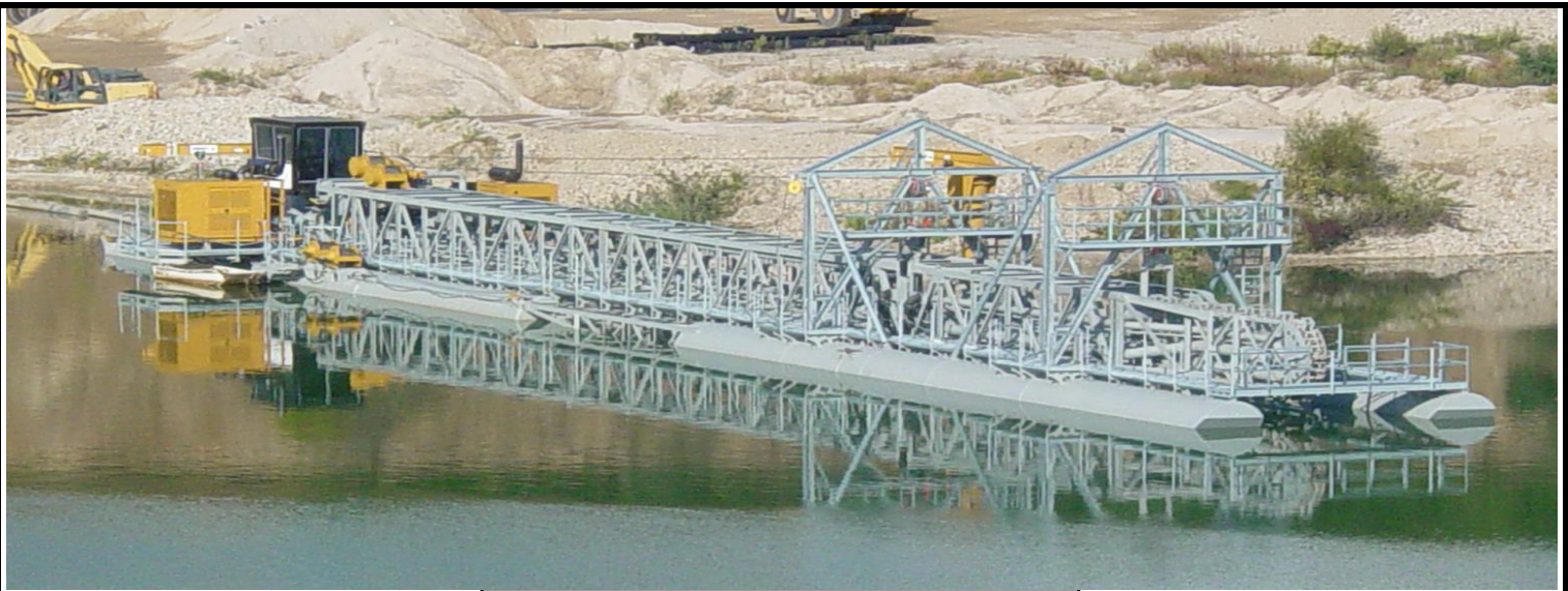
L-Series PELICAN dredge with diesel power
