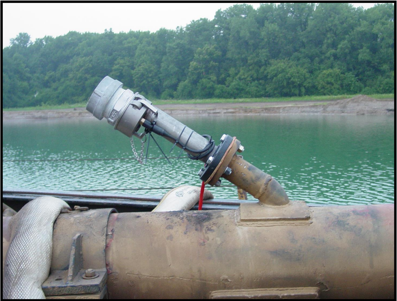
Twinkle Co LADDERVAC II inlet sensor mounted on the suction pipe of a ladderpump dredge.
