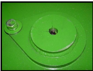
Extreme-duty shaft with recessed grease zerks.
