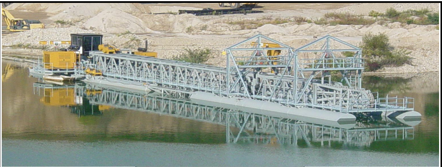
L-Series PELICAN dredge with diesel power
