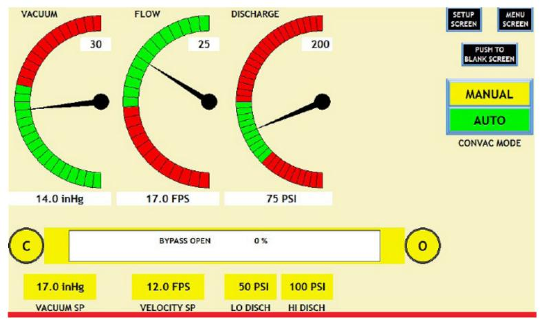
The CONVAC S4 Suction Side Stability System combines the LNV bypass valve with a new and improved control system. CONVAC S4 allows for unprecedented control of the dredge system variables which results in improved production, constant flow and reduced production costs. Features of the new control system include:
