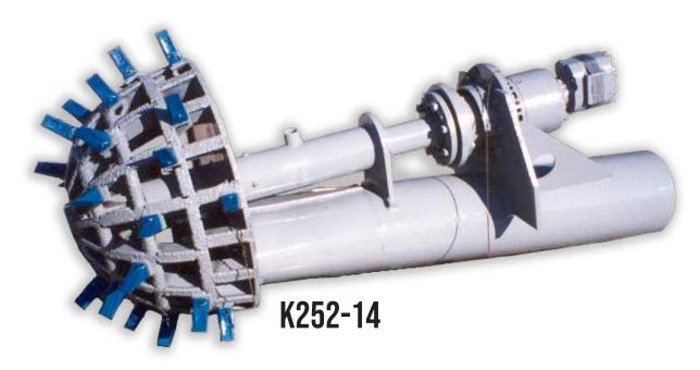
Twinkle Co K3 & K252 cutterheads are the ideal choice for most sand & gravel dredging applications. Both the K3 & K252 feature a hydraulic motor, oil-filled sealed planetary gearbox, drive coupling, 4.5" driveshaft, marine bearing and bolt-in bearing tube, tapered basket mounting, and 3" basket retainer thread. Twinkle Co cutterhead assemblies are mounted on a length of suction pipe and ready for installation on your dredge. A static oil head tank and basket nut wrench are included.
