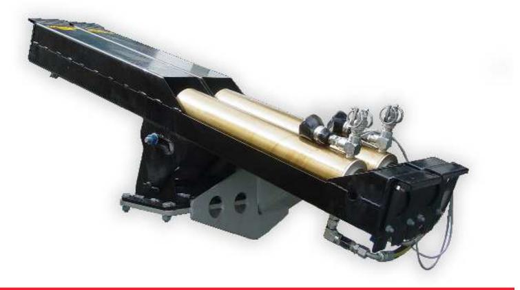
Dynamic Head Tanks – A simple way to maintain pressure in a sealed housing. Maintaining a positive internal/ ambient pressure differential is critical for a sealed housing operating underwater, such as a ladderpump bearing housing or a cutter drive gearbox. A positive differential is created when the internal housing pressure (head) is greater than the external water pressure. Failure to maintain a positive differential will allow water intrusion and lead to failure.
