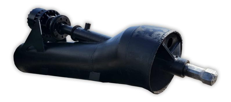
The rugged, lightweight, powerful MUZZLELOADERS attach directly to the end of the suction pipe. What was a smooth-mouthed, plain-suction pussycat of a dredge is now tearing up a Wisconsin pit with an 8-inch MUZZLE-LOADER at a rate the owner claims to be three times as much as the plain suction! Now there is plenty of sand and gravel—no oversize-ready to pump all the time.
