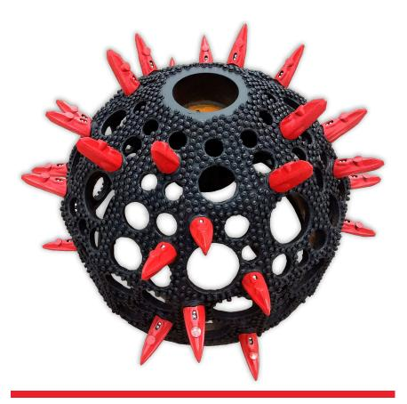
The surface protection on a standard Claymator basket is a pattern of wire-weld hardfacing. For severe duty applications the hardfacing may not provide adequate service life and a more robust type of surface protection is required. The severe duty solution is CLAYMATOR Heavy Metal that covers the surface with carbide buttons.
