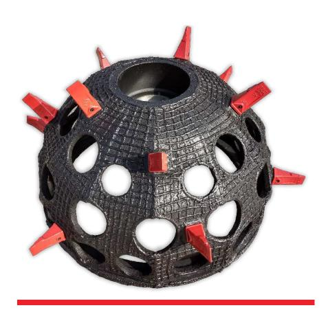
The unique design of the CLAYMATOR "screens and cleans" as it rotates. The openings are designed and arranged to reject oversize material and scrub away clay. This allows for continuous, uninterrupted and profitable operation. The CLAYMATOR cutter has individually replaceable teeth and is bi-directional.
