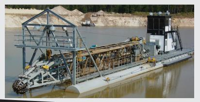
Deep depth mining dredges with pump discharge sizes from 8" to 16"
