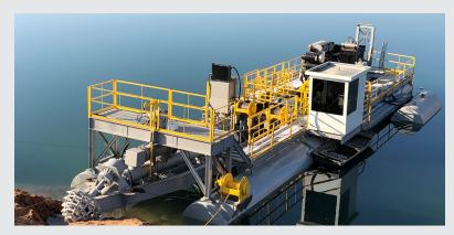
Shallow to medium depth mining dredges with pump discharge sizes from 8" to 16"
